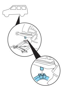
3. Position the jack according to the guides and turn the jack handle clockwise until the tire is a maximum of 1 inch (25 mm) off the ground.
